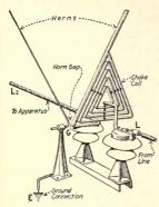
Fig. 169.—Horn-gap, choke-coil protector for alternating-current lines.
